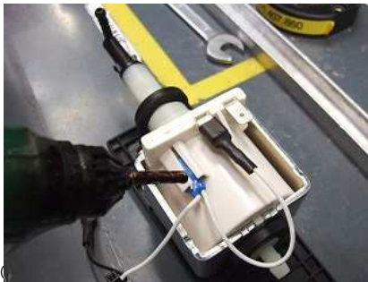
Apply 0.38 grams of hot glue in both side sides, out of the slit of the thermal protector (see Pict. 2 and Pict. 3)
