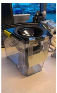
Per wk. 1314 the tapes are added during assembly of the appliances
