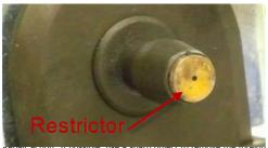
Acpair action. It possible, use a snarp object to remove the foreign material blocking the restrictor opening.
