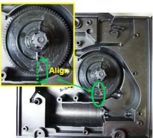
2. The gear, pn 14002800, has to be the one with "2" printed on the top (see picture nr 2). Make sure you have the right part, otherwise, order the kit 421941307001
