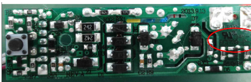
Generation 2 Power PCB 996510073641 Identification (Printed with EC1739-P-21 on the PCBA)
