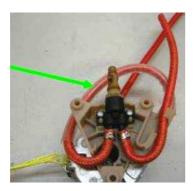
Royal Professional: Insert a new red tube (L = 240 mm; part code: 11000756) from pump to boiler positioning it correctly in order to avoid bending, and insert also a new transparent tube (L = 200 mm; part code: 9972.166) from the safety valve to the discharge in the drip tray as shown in the picture 3.
