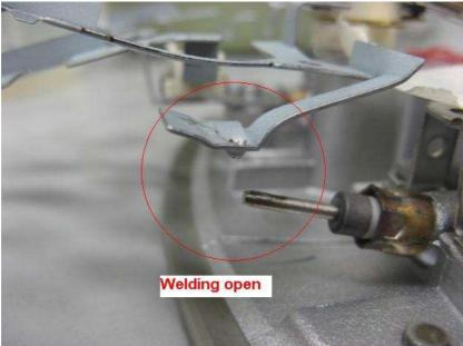
**CURE:**For service repair, please replace the complete soleplate assy. It is not possible to do the welding at service center because specialized equipment & process control is required for the spot welding process.
