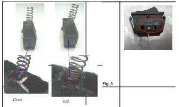
**<u>Cure</u>**: Replace Display Panel printed assy (Position 47). In this manner, affected switch module replaced.
