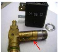
Please replace the defective electro-valve. Service code: 4239 017 10901.
