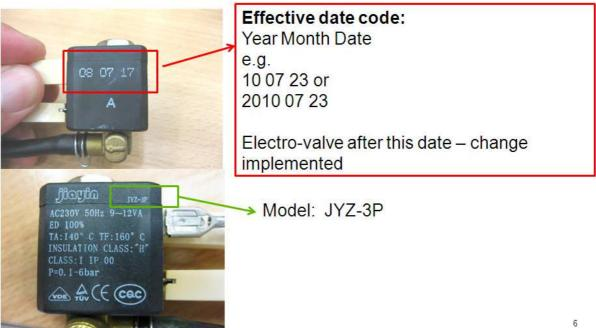
In addition, below picture shows the difference between the new part & the old part.
