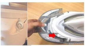
Cure: Replace CEME e-valve with Jiayin valve Electrovalve (90 deg) - diagraphm 4239 017 11581
