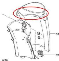
CURE: Replace any defective or malfunctioning water container with the supplied one, if possible or preferred, transfer the cover from the original Water Container.
