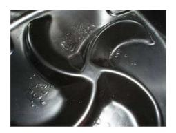
**Symptom 2.** Coating layer wear off due to abrasion from Basketholder (Pan)
