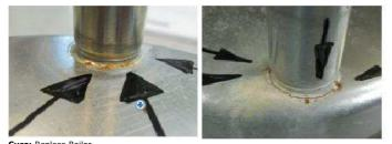
Cure: Replace Boiler After replacement, Check to ensure no leakage of steam by placing a mirror next to collar (e.g. to see any condensation formed on mirror)
