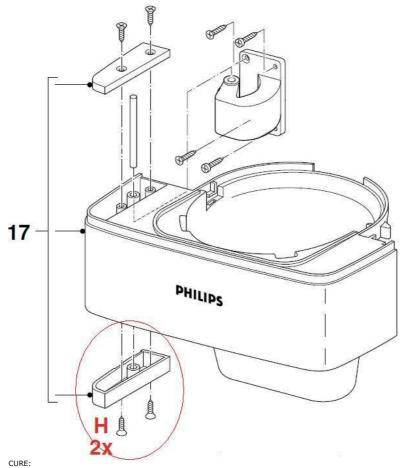
CURE: When you receive the spare from DHL, please transfer the cover and screws from the original filterholder to the new spare filterholder.
