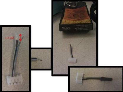
Please note: For Senseo Viva Cafe and Senseo Quadrante: These models have a hall sensor to detect the brewhead being closed. Here only wires 1 and 2 need to be solderded together, otherwise the power supply will be short circuited and the appliance will not start up. The brewhead sensor for Viva Café has a 3 pin connector, the sensor for Quadrante has a 4 pin connector. on the side of the receptacle the first pin is indicated by a "1".
