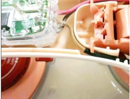
All GC36xx and GC37xx (ASO version) product returns for servicing is required to re-dress the ASO wires according to the symptom cure, regardless of complaint symptoms.
