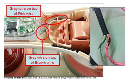
Symptom Cure: Replace ASO (4239 021 56033) and ensure the ASO wires dressing is correct, as shown below.
