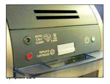
When the red REPLACE CARTRIDGE light starts flashing and beeping, it is necessary to continue steaming for at least 10 minutes, ignoring the flashing and beeping. This will allow the system to register the hard water. Then, replaces the anti-calc cartridge and continues to steam for at least 10 minutes to allow the system to register soft water. Once the system successfully registers hard water and soft water in sequence, ACC will activate upon the next start up.
