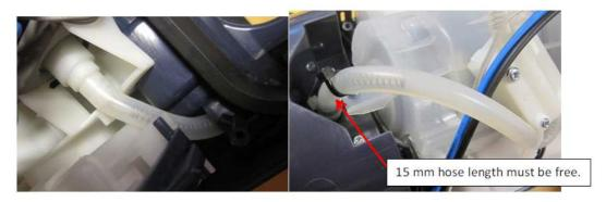
Add a spring to the water hose from the clean water tank outlet to the water sensor.
