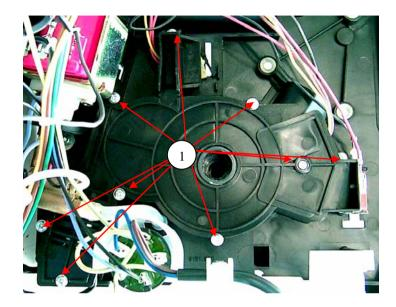
f) Unscrew the nine screws (1) of the gear cover and remove cover.
