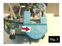
• Remove the thermo isolation of the tube heater.
