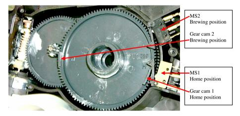
Note: The gear wheel must always be installed so that MS1 and MS2 are positioned at the long section of the switching cams!
