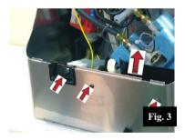
• Pull the switch off the seat and loosen the two screws as shown in the figure.
