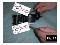
• In case the sprocket is worn out, remove the gear, by means of a 7mm and a 10 mm fork wrench.
