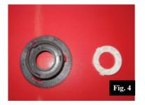
• Press the release button (1) and at the same time turn the ring nut (2) counterclockwise to the end of its stroke and remove the ringnut.
