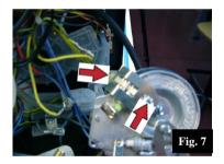
• Remove the mounting screw of the sensor hoder and remove the sensor.
