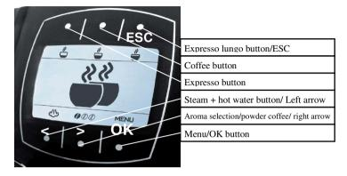
Access: Access from the standby mode (press MENU/OK) by keeping the EXPRESSO and HOT WATER button pressed, whilst pressing briefly the ON button. From Version: 2.00.1
