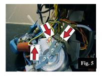
• Remove the three faston connectors, as shown in figure 5.
