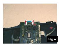
• Remove the blue flat cable as shown in the figure.
