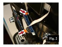
• Remove the two flat cables.
