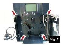
• Remove the four screws, as shown in the figure.
