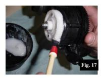
• Grease the sprocket.
