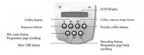
Access: Access from the standby mode (press 2x Menu/OK) by keeping the EXPRESSO, LONG COFFEE and HOT WATER button pressed and pressing the MENU/OK button with a slight delay. (The user programme is also available in this mode.)
