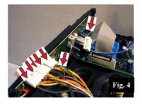
• Remove all connectors of the electronic board.
