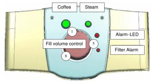
Various test functions can be activated in the service mode by activating either the coffee or steam buttons in conjunction with various coffee quantity settings.
