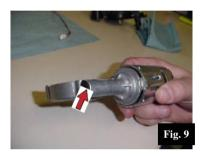
• Fit the rubber cap to the flange of the new grinder motor.
