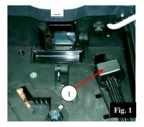
• Remove the measuring scoop.
