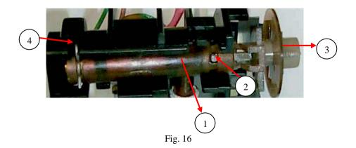
e) Remove valve components from housing.
