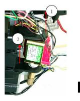
• Seperate the upper Pump support (1) from the pump and the lower pump support (2) from the support plate.
