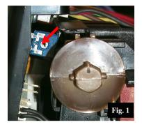
• Remove the HWS-knob and adjust the dosage as follows: Rotation counterclockwise decreases dosage (min 6 grammes) Rotation clockwise increases the dosage (max 10,5 grammes).
