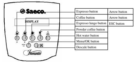
Access: Access from the standby mode (press 2x Menu/OK) by keeping the EXPRESSO, EXPRESSO LUNGO and HOT WATER button pressed and pressing the MENU/OK button with a slight delay. (The user programme is also available in this mode.)
