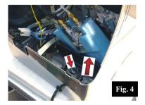
• Remove the cable compartment, as shown in the figure 4.
