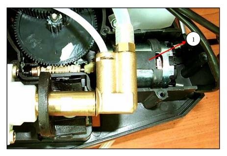
The gear motor can be removed without dismantling the pump (1).
