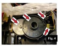
• Remove all the screws from the gear motor cover.
