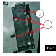
• Unlock the four (three) notches, and remove the locking plate.
