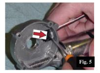
• Remove the sensor, by pressing the anchoring tab by means of a screwdriver......
