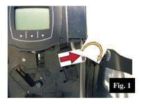
• Remove the steam tube connection by pulling while rotating counter clockwise.
