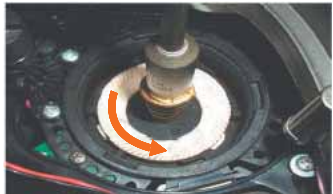
On the lower burr, keep the increment pin as indicated locked in position and proceed as shown in the figure above.
