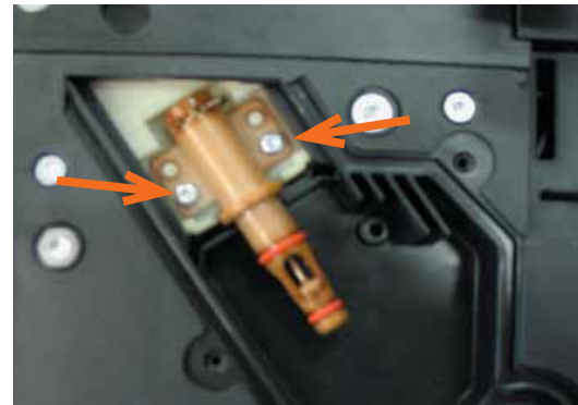
Loosen the two screws and remove the boiler valve (B).
