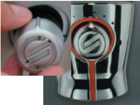
Remove the knob with the Saeco logo by pulling outwards.
