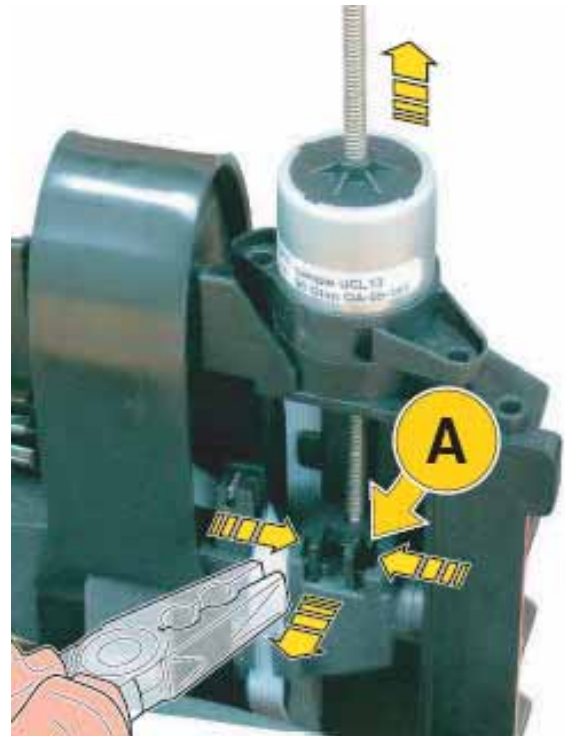
To withdraw the stop (A) use pliers to grip the tabs securing the lifting system to the base and pull outwards. Withdraw the brew drive with worm gear from above.
