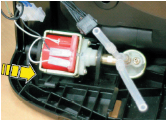
Withdraw the silicon tube that comes from the turbine.
