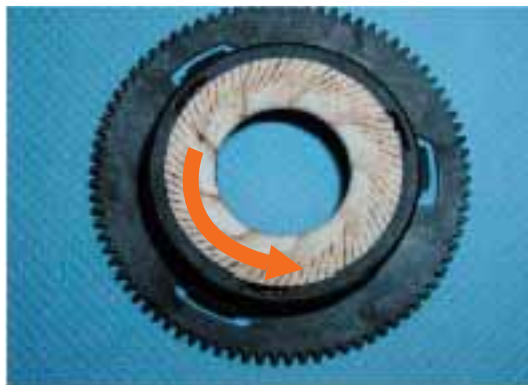
To remove the upper burr, rotate anti-clockwise until it detaches from the bayonet coupling.
