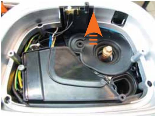
Remove the coffee container and rubber seal.
