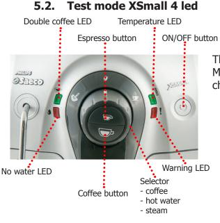
This document describes the test mode of XSmall Evo Machine. This application is used in order to test the machine in its mechanics and electronic components.
