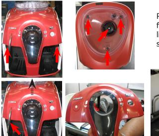
Remove the dreg drawer, water tank, mushroom finger protection device on the coffee container lid and coffee container, then loosen the screws shown.
