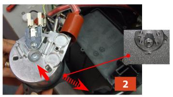
**2**) Loosen the screw and remove the plastic support. Disconnect the hoses and the connections.
