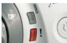
Brew group is not inserted. Coffee ground drawer is not inserted. Service door is open. Control dial is not in correct position.
