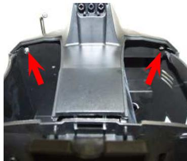
Remove the dreg drawer, water tank, mushroom finger protection device on the coffee container lid, then loosen the screws shown.
