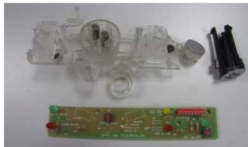
To remove the coffee keys from the control keypad, detach them from the anchoring device on the back of it and take them out.
