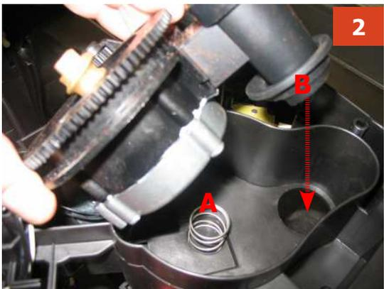
**1)** To remove the coffee grinder, simply slide it out and remove its connections.
