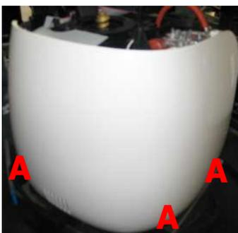
Loosen the screws shown and slide out the side cover; be careful of the protrusions **(A)** on the base.
