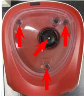
Remove the dreg drawer, water tank, mushroom finger protection device on the coffee container lid and coffee container, then loosen the screws shown.
