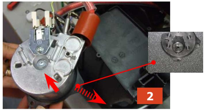
2) Loosen the screw and remove the plastic support. Disconnect the hoses and the connections.
