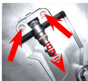
Loosen the screw and remove the boiler pin.
