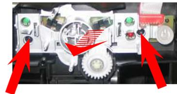
Loosen the screw and remove the control knob and coffee keys.
