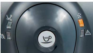
Machine is dispensing descaling solution
