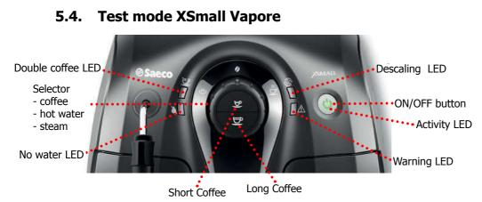
This document describes the test mode of XSmall Vapore. This application is used in order to test the machine in its mechanics and electronic components.
