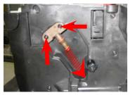
Loosen the screws shown and remove the boiler pin.
