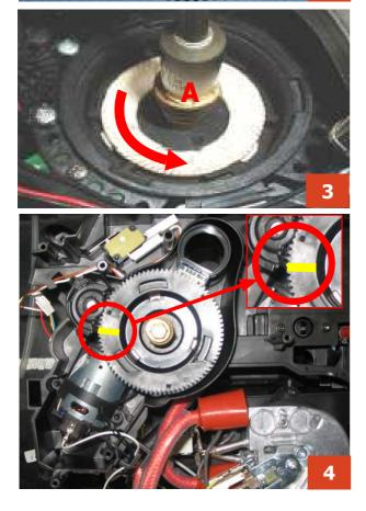
**3)** To remove the lower grinder blade, keep the increment pin (A) locked in position and turn the grinder blade anti-clockwise, until it detaches from the bayonet coupling
