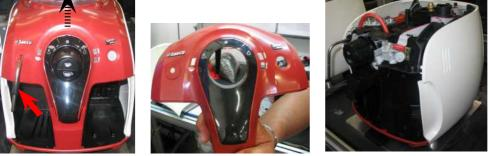
Slide out the steam hose protection, lift the cover at the rear by pressing down gently on the cooling vents to help detach the anchoring tabs, then pull it away from the steam hose, taking care not to scratch it.
