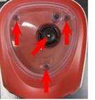
Remove the dreg drawer, water tank, mushroom finger protection device on the coffee container lid and coffee container, then loosen the screws shown.
