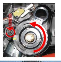
**1)** To remove the upper grinder support, using a hex key push down and turn clockwise to release the grinder support from the bayonet coupling
