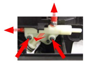
Loosen the screw and disconnect the hydraulic connections, remove the flow selector faucet.
