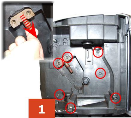
1) Loosen the screws holding the boiler pin in place, remove it and loosen the other screws shown
