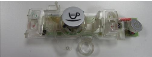
To remove the coffee keys from the control keypad, detach them from the anchoring device on the back of it and take them out.
