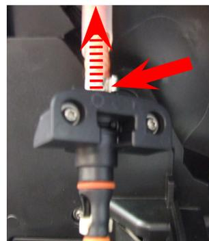
Remove the OETIKER clamp and pull out the silicon tube
