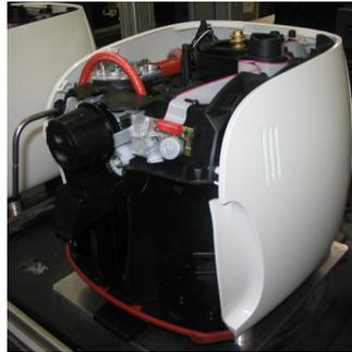
Slide out the steam hose protection, lift the cover at the rear by pressing down gently on the cooling vents to help detach the anchoring tabs, then pull it away from the steam hose, taking care not to scratch it.
