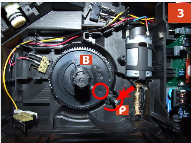
3) Replace the gear (B), making sure that the imprint of the arrow is aligned with the opening containing the pin (P)
