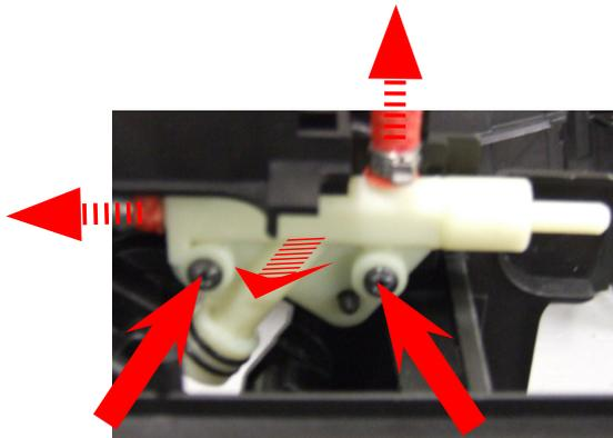
Loosen the screw and disconnect the hydraulic connections, remove the flow selector faucet.
