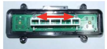
Loosen the screws as shown
