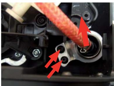
Loosen the screws to remove the steam pipe
