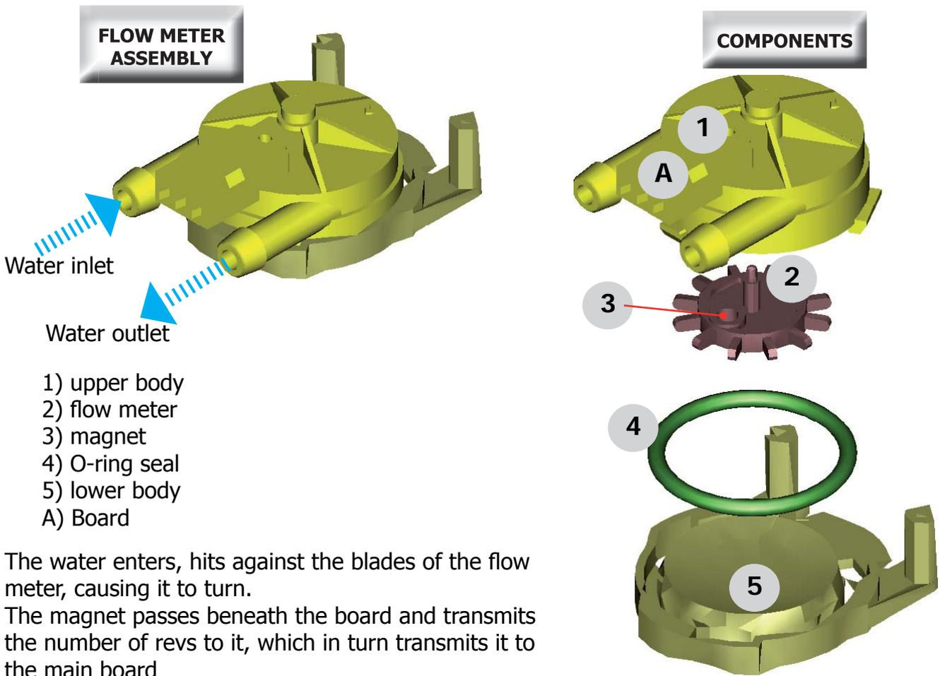
The water enters, hits against the blades of the flow meter, causing it to turn.
