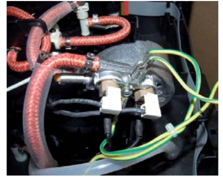
Remove the water and electric connections
