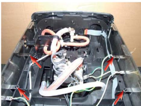
Loosen the screws as shown
