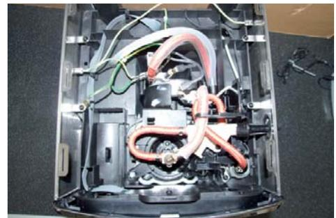
Loosen the screws as shown on the rear part of the machine and lift the cover
