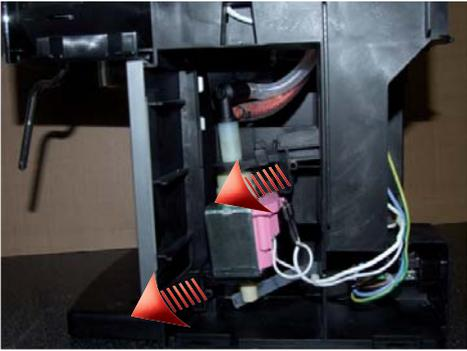
Remove the pump from the supports as the picture
