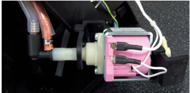
Remove the water and electric connections
