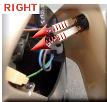
RIGHT side cover. Remove the connection of the on/off switch from the cover
