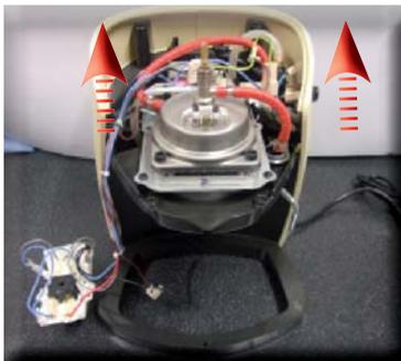
Remove the side covers by lifting them upwards
