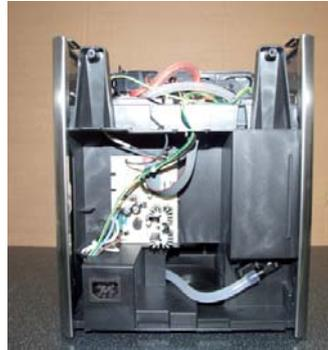
Remove the posterior cover lifting it upwards
