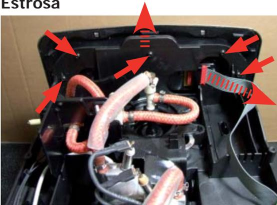
Loosen the screws, the electric connection and remove front panel as shown
