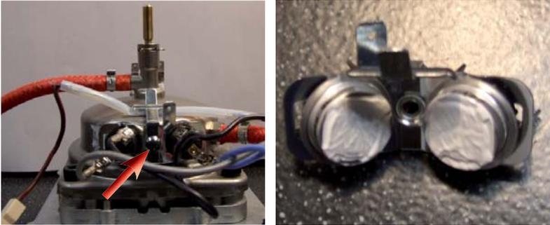
When putting back the thermostats, always apply conductive paste for the thermostat to adhere perfectly to the boiler
