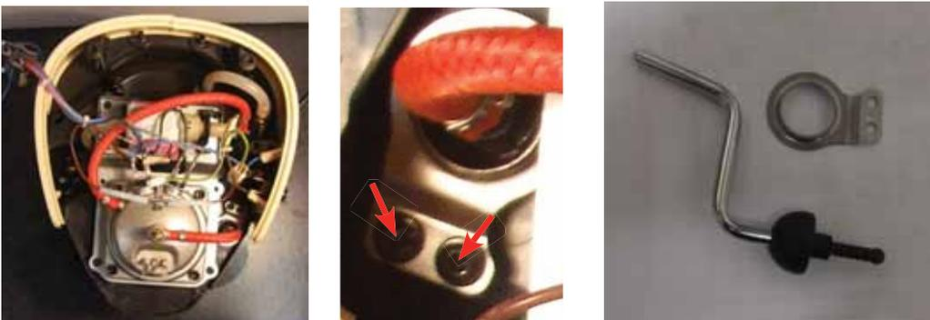
Loosen the screws as shown
