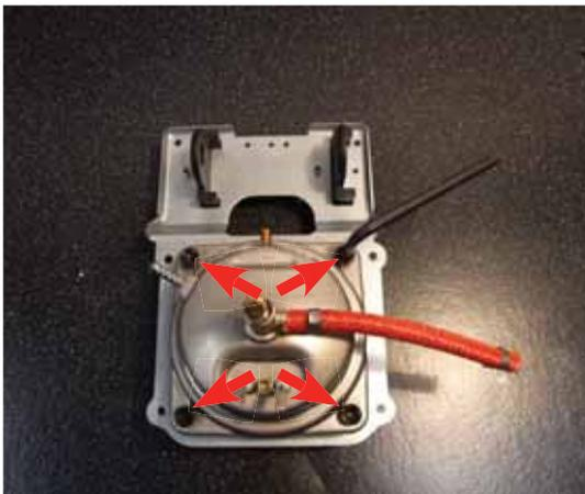
Loosen the screws as shown
