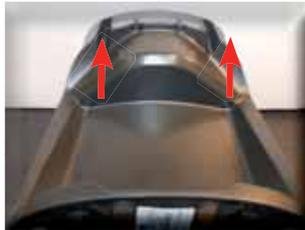
Loosen the screws as shown on the front and rear part of the machine
