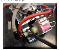
Loosen the overpressure valve
