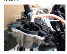
Remove the water connections
