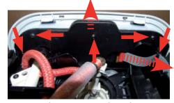
Loosen the screws, the electric connection and remove front panel as shown
