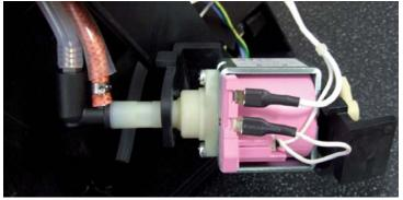
Remove the water and electric connections
