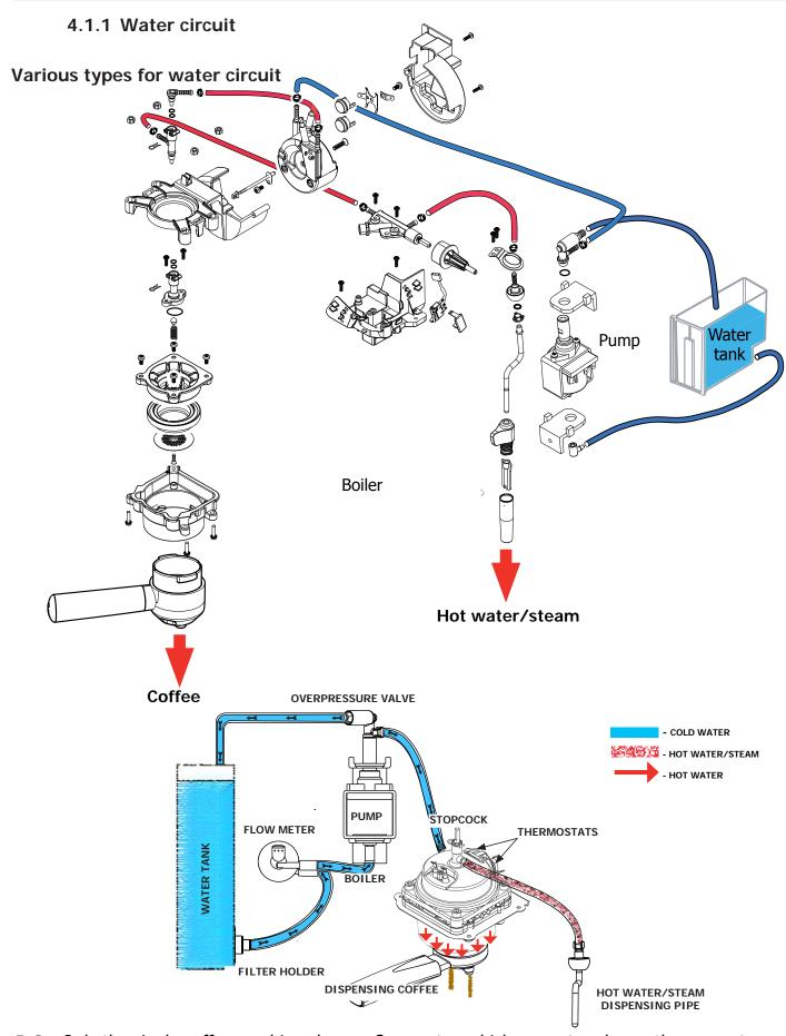
**P.S.**: Only the single coffee machines have a flow meter, which can set and save the amount of dispensed coffee via the control board.
