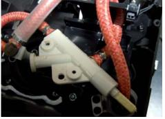
Remove the water connections
