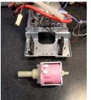
Remove the pump from the supports
