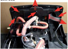
Loosen the screws, the electric connection and remove front panel as shown
