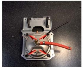
Loosen the screws as shown
