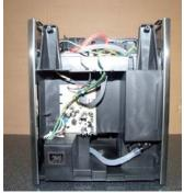
Remove the posterior cover lifting it upwards
