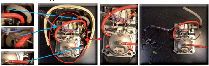
Remove the water connections and loosen the screws as shown
