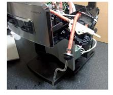
Loosen the screws to remove the steam pipe
