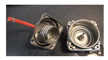
Check the internal condition of the boiler (limescale, any breakages, condition of the O-ring seal, etc.)
