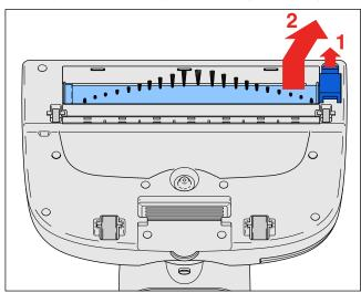
To place the Brush, position the Brush over the Roller Holder assy (13) then "click" the Brush into place at the Roller Brush cover and close the Roller Brush cover.
