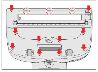
To replace the pump (10): First remove the Water Tank (3) and Filter assy (4). Remove the 4 screws (C), and remove the cover. Now the pump is visible. Remove the clips from the hoses and the valve and replace the pump.
