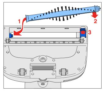
To replace the Brush Motor (15), Driving belt (12) and Roller Holder assy (13): Remove the 10 screws (D) on the bottom of the Nozzle and push the 3 clicknocks on the front side with a screwdriver, now the components can be reached.
