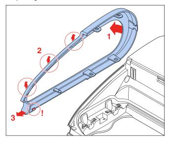
Carefully unsnap the collar from the nozzle. Next remove 11 screws L (2 are underneath the collar) to be able to remove the upper housing from the nozzle.
