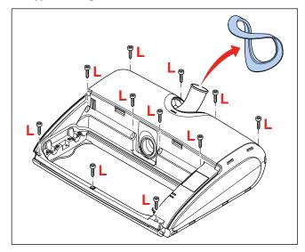
You can now easily access all components like the Nozzle PCBA, pump, suction tube, drive train etc.
