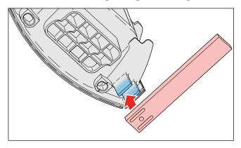
• Drill a  $\emptyset$  2.8 mm hole, through the cutting plate, in the housing rear.
