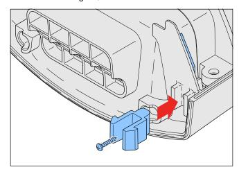
• Tighten the screw. Make sure the bottom of the click finger 4 touches the housing rear. If not, most likely the remaining leg(s) are still to long.
