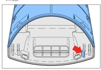
• Place the (drilling and) cutting plate. With the chamfers of the holes for the legs facing the housing rear.
