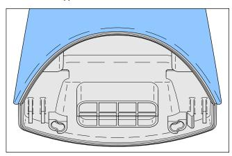
• Remove the housing front (and if needed the remaining click(s)).
