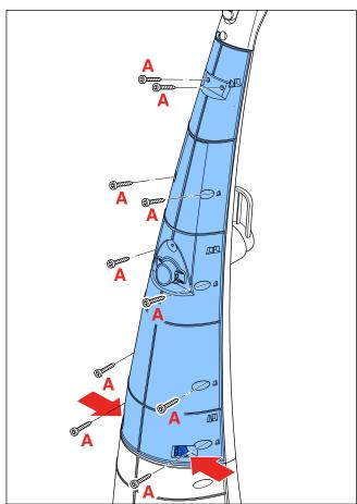
Secondly remove the ten screws  $\mathbf{E}$  from the Front Frame and remove the Front Frame from the Lower Stick assy. You can now access all internal components.
