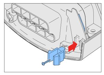
• Tighten the screw. Make sure the bottom of the click finger 4 touches the housing rear. If not, most likely the remaining leg(s) are still to long.
