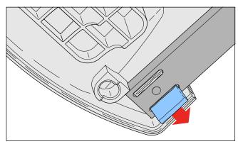
• Remove the second leg. Make sure the cutted surfaces of the legs is not sticking out the plate. If needed, adapt this by cutting or filing the legs.
