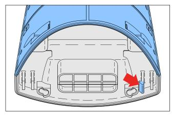
• Place the (drilling and) cutting plate. With the chamfers of the holes for the legs facing the housing rear.
