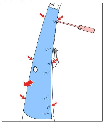
To remove the decorative cover of the lower stick, take a small flat-head screwdriver and unlock the eight snaps as indicated in the illustration below. Carefully move the panel forward, there are eight pillars guiding the panel on the frame behind.
