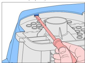
• To replace the parkhook (13), first remove Screw C, then by pushing the two lips with a screwdriver the parkhook can be removed (see picture).
