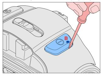
Finally the last screw B that need to be removed is situated at the bottom side of the appliance (see picture).
