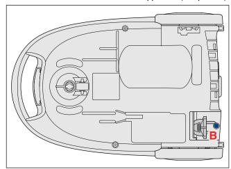
To separate the top housing from the bottom housing release the snap connection behind the wheel at the cordwinder side (see picture).
