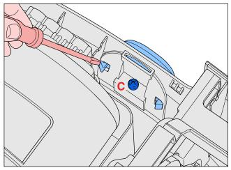
• To replace the cordwinder (20), first remove the wires, the locks can be unlocked with a screw driver (see picture).
