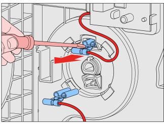
• The safety valve assy (21) can be clogged with dust, it can be easily taken out and replaced after the tophousing has been removed, it must be done from inside the bottom housing where the cordwinder is situated (see picture).
