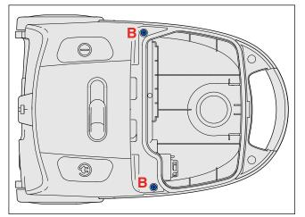
• The 3<sup>th</sup> screw **B** is hidden under the On/Off pedal (12), to remove the pedal use a screwdriver (see picture).
