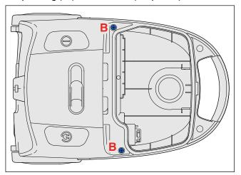
• The 3<sup>th</sup> screw **B** is hidden under the On/Off pedal (12), to remove the pedal use a screwdriver (see picture).
