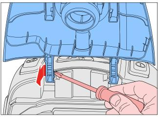
• When the dustcover has been removed, 2 of the 4 screws **B** that need to be unscrewed to disassemble the tophousing (**15**) are accessible (see picture).
