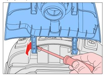
When the dustcover has been removed, 2 of the 4 screws B that need to be unscrewed to disassemble the tophousing (15) are accessible (see picture).
