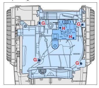
• To replace the PCB (9) remove the 2 short screws H.
