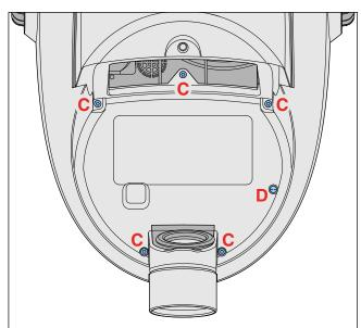
To replace the potmeter (9) situated at the bottom
