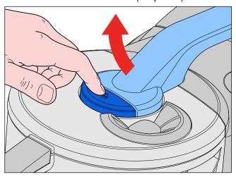
The button (3) on the lid is a spare part, it can be replaced by removing screw A (see picture).
