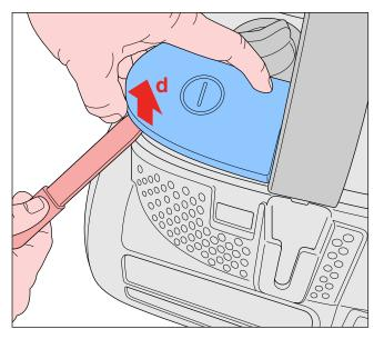
• When assembling, the buttons can easily be mounted by clicking, start at the side of the handle.
