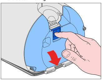
To reach the inner parts for repair, Upper housing (18) has to be removed. First the On/Off button (17) and Cordwinder button (16) must be removed, this can be done with a screwdriver.
