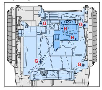
• To replace the PCB (9) remove the 2 short screws H.
