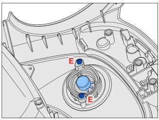
After removing the Upperhousing, Hose connection (10) and Bucket inlet sealing (13) are accessible. To replace the Hose connection screw F has to be removed.
