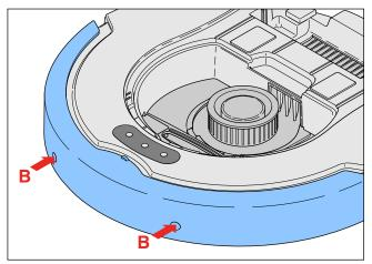
After removing the front bumper turn the appliance upside down on a clean surface and remove the 6 screws
