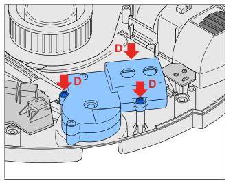
• The PCB main (14) is a complete assy, and can be replaced. A screwdriver can be used to remove the connectors. (see picture)
