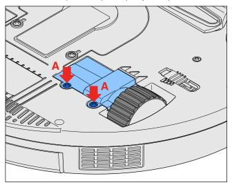
• Disconnect the connector and replace the wheel set.
