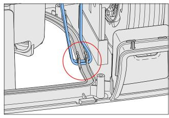
The frame that holds Triple filter (18) is attached to the Upper housing, to remove the frame remove screw
