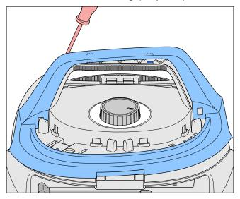
Remove the 2 screws A which hold Handle (9) and screw B (see picture).
