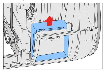
• When assembling take care that the wires from motor to cordwinder are correctly fixed (see picture).
