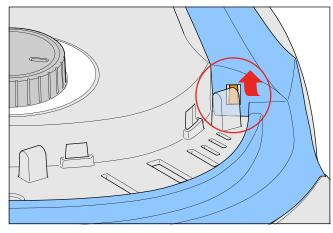
• Now you can with a screwdriver remove the complete Handle cover from the housing (see picture).
