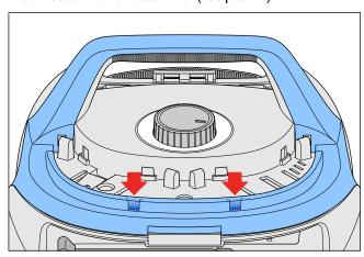
• Then with a small screwdriver lift the Handle cover over the nock on the Top housing (see picture).
