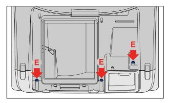
When replacing the Cordwinder (21) the Lower housing insert (19) needs to be removed. Move the Lower housing insert upwards so the cordwinder can easily be removed (see picture).
