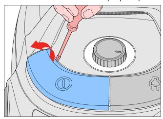
• To remove Handle cover (8) first release the 2 snap connections on the backside (see picture).
