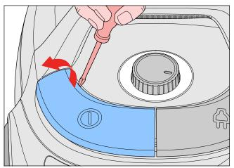
• To remove Handle cover (8) first release the 2 snap connections on the backside (see picture).
