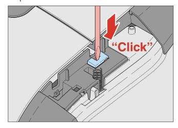
Finally re-assemble the button. Press it firmly, until the "Click".
