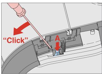
To prevent lever shifting out of position to re-occur, CW support (Pos. 68) must be added as shown in below pictures:
