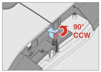
Then drop the part till it is completely inside the appliance and push down with a screwdriver untill "Click".
