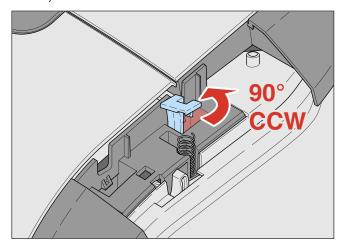
Then drop the part till it is completely inside the appliance and push down with a screwdriver untill "Click".
