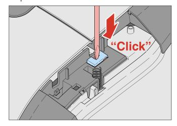
Finally re-assemble the button. Press it firmly, until the "Click".
