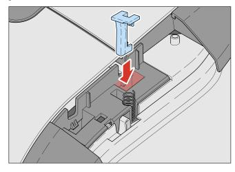
Rotate the part 90 degrees CCW, once it is inside the housing half way.
