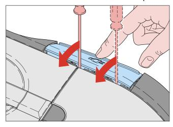
Remove the cord winder button by simultaneously operating the button and putting a screwdriver between the openings that occur.
