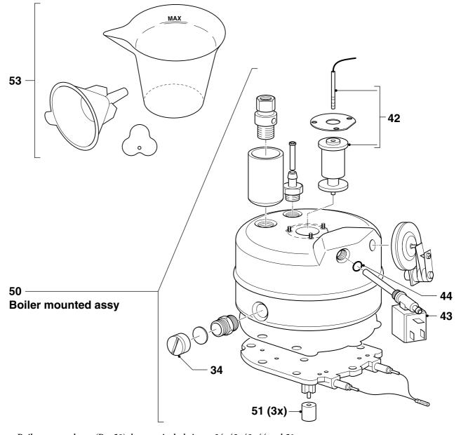
Note: Boiler mounted assy (Pos 50) does not include items 34, 42, 43, 44 and 51
