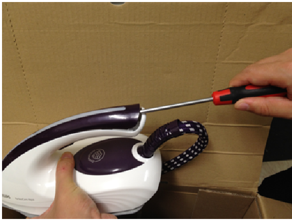
Fig 1 Using "-" screw driver to lift up the Inlay and release the catch at the end of the handle
